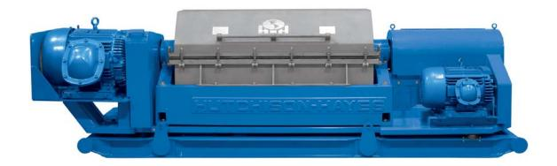
The HH 5500 CentriSmart is a configuration of a drive system for a Decanting centrifuge with infinite variability options on the conveying speed. This configuration is a fully variable speed selection of bowl speed and conveying speed. The Centrifuge bowl is driven by a main drive motor and the conveyor is driven through a planetary gear box by a back-drive motor, both controlled by PLC and speed selection through Variable Frequency Drives.
