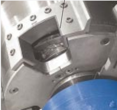
Tungsten Carbide wear protection for erosive applications
